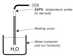
Check periodically the sock installed on the sensor has not been clogged by calcium carbonate scale. If so, remove it then clean or replace it.
